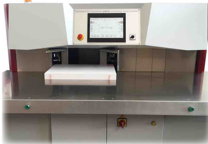
STAINLESS STEEL BLOWING TABLE AND PROTECTION GUARD
