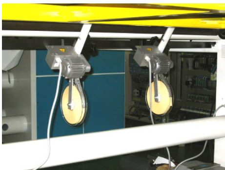
Configuration with 2 tab-inserter with single roll with rear application to sheeter.
