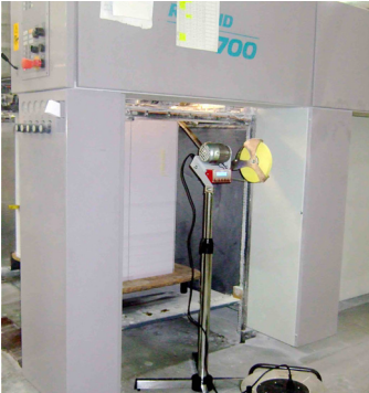
Application on printing machine - Rolad with lateral insertion.
